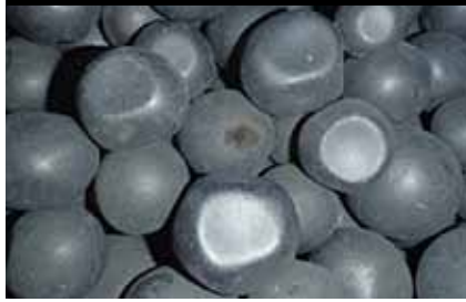
Figure 7: low-quality media in the first chamber
