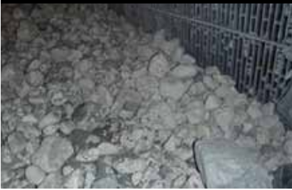
Figure 6: over-sized material in the first chamber
