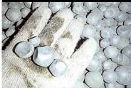
Figure 9: low-quality media in the second chamber
